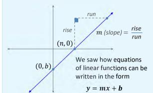
Where m is the **slope** of the line, and b is the y-intercept
